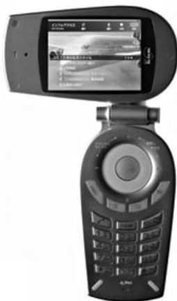
Figure 4. Prototype Mobile Phone Handset Equipped with a Function to Receive Mobile Phone Broadcasts
